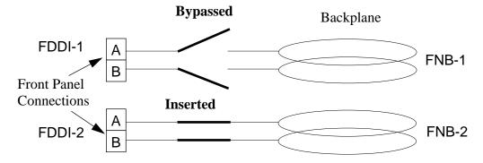
Figure 1. Front Panel Connections "Inserted" and "Bypassed"
